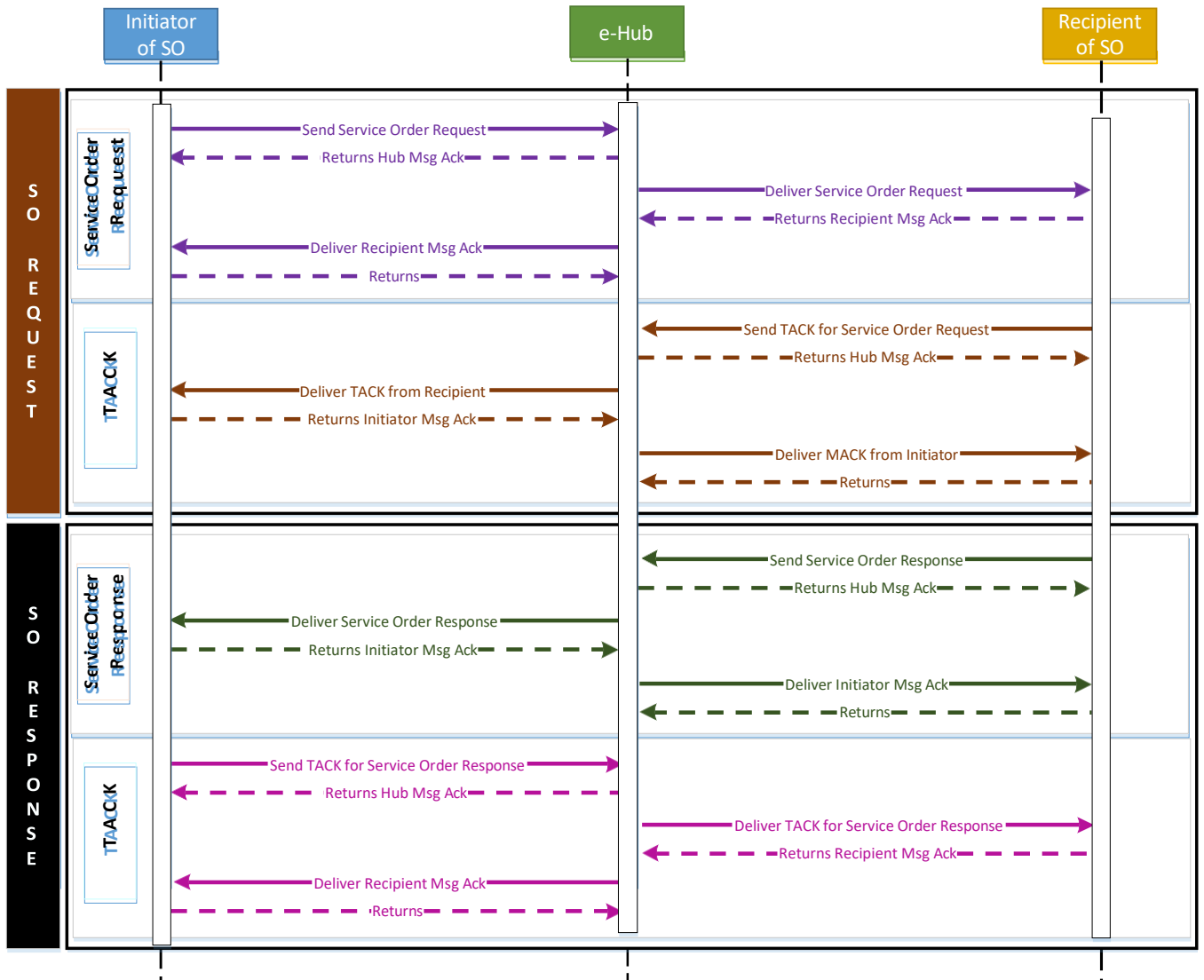
Figure 15 Example of Webservices Transaction Model for Service Order process
